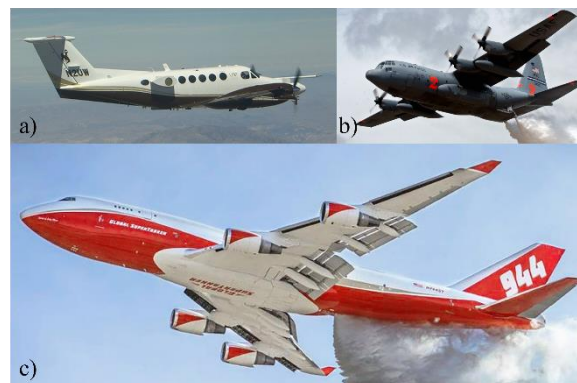
Figure 1. All aircraft under study. (a) University of Wyoming's King Air 350 used for meteorological testing. (b) Converted C-130 using a MAAF's firefighting system. (c) Global Supertanker Service's Boeing 747-400 firefighting air tanker.
