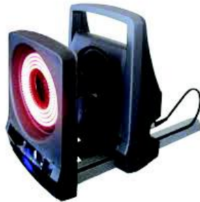
Figure 3-2. Vicon T40s camera with strobe on. Image source: svga.ru.
