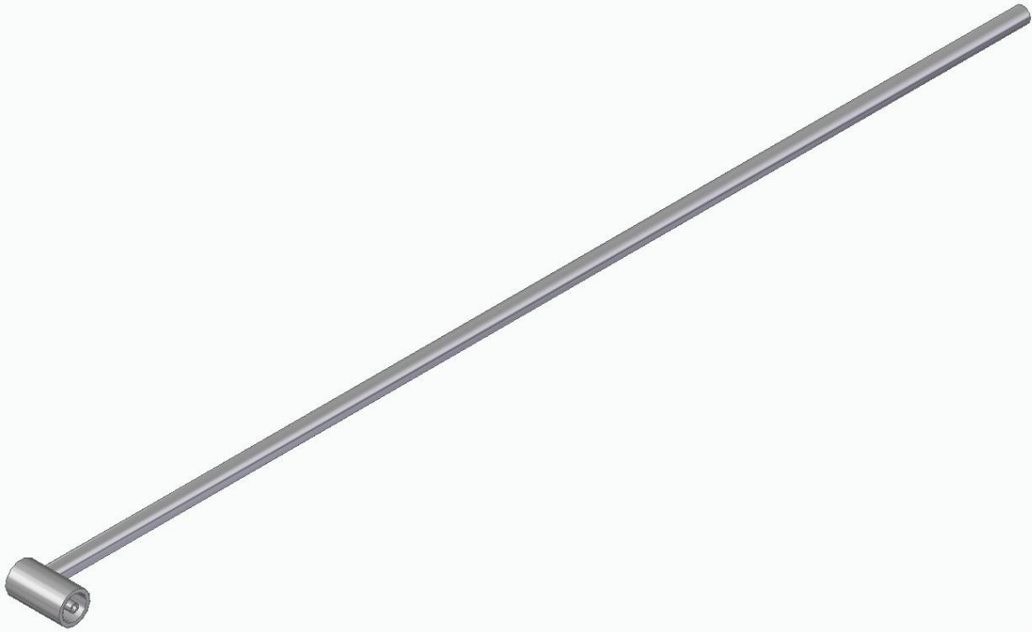
Figure 19. Three-dimensional isometric view of the KCC-8 Kiel probe.
