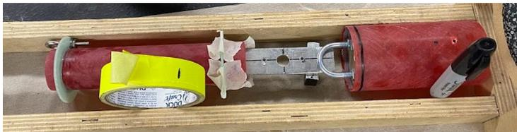
**Figure 5 Curing Orientation for Motor Mount Tube and Nose Cone Coupler**
