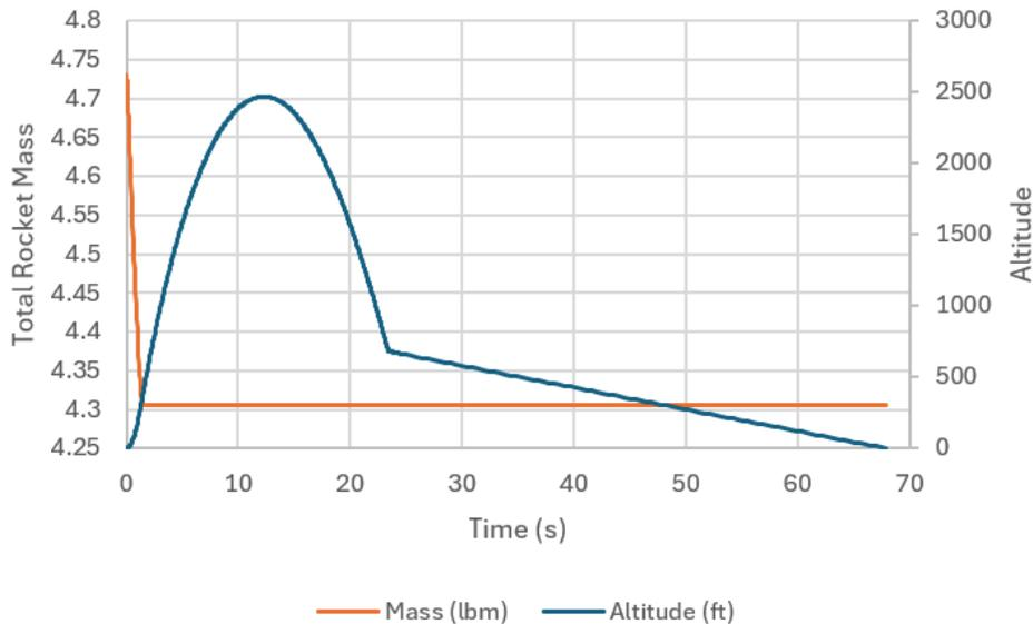
Figure 21 Second Altitude and Total Rocket Mass Profile for I-218
