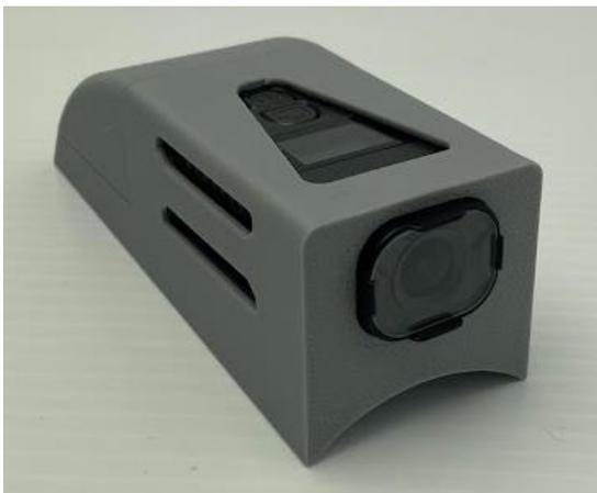
**Figure 15 RunCam 6 Installed in Shroud**
