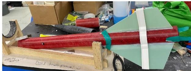
**Figure 8 Curing Set Up for Lower Airframe Assembly**
