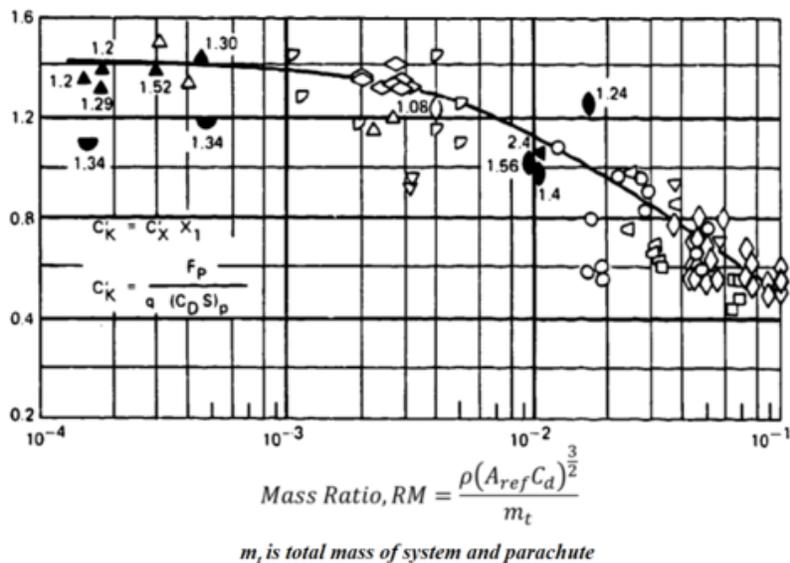
Figure 17 Opening Force Factor vs. Mass Ratio
