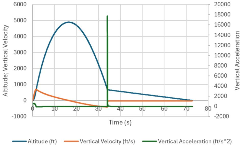
Figure 24 Final Altitude, Velocity, and Acceleration Profile for J-420
