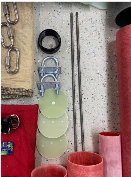
**Figure 3 Bulkheads, U-Bolts, All Threads, and Motor Retainer**
