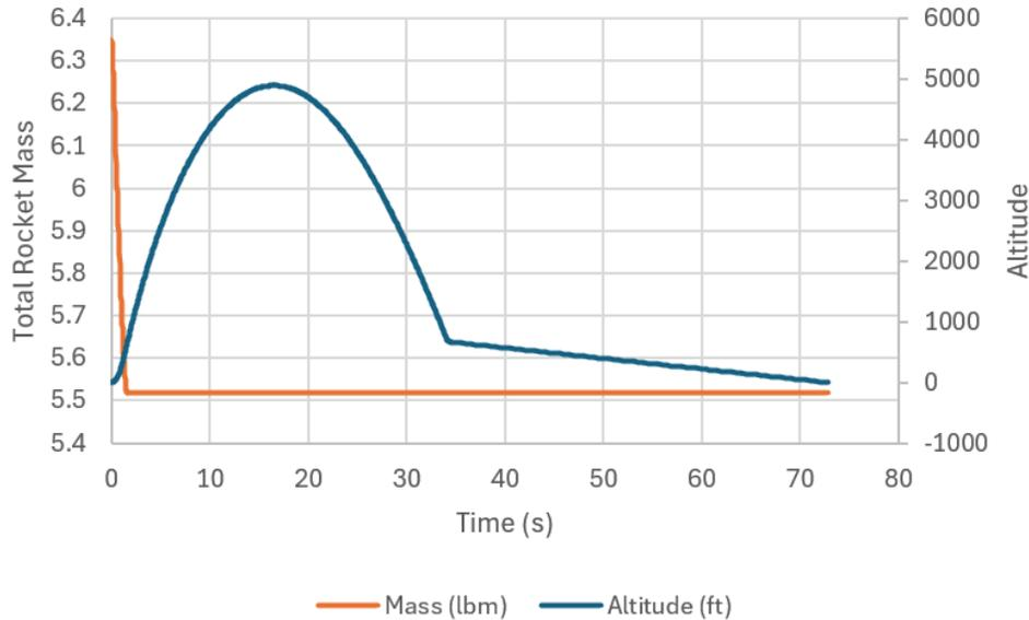
Figure 25 Final Altitude and Total Rocket Mass Profile for J-420
