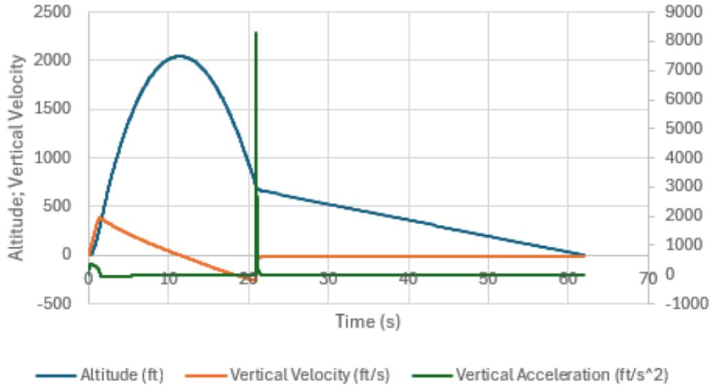
Figure 18 Initial Altitude, Velocity, and Acceleration Profile for I-218
