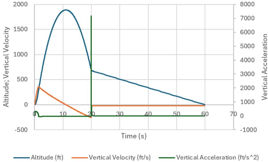
Figure 22 Final Altitude, Velocity, and Acceleration Profile for I-218
