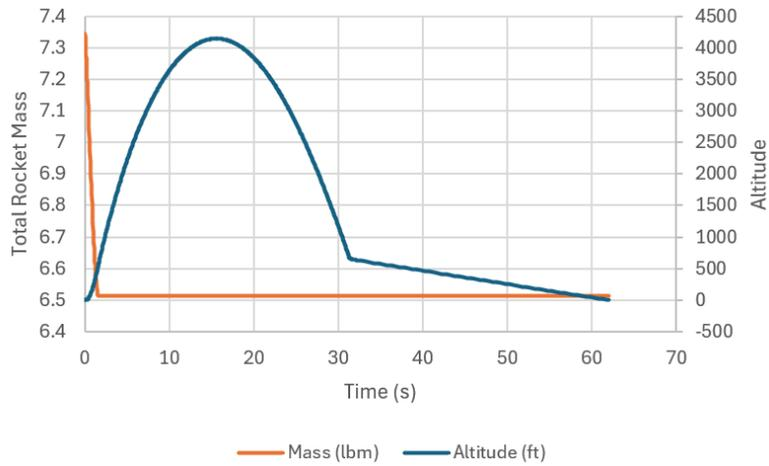
Figure 35 Initial Altitude and Total Rocket Mass Profile for J-420
