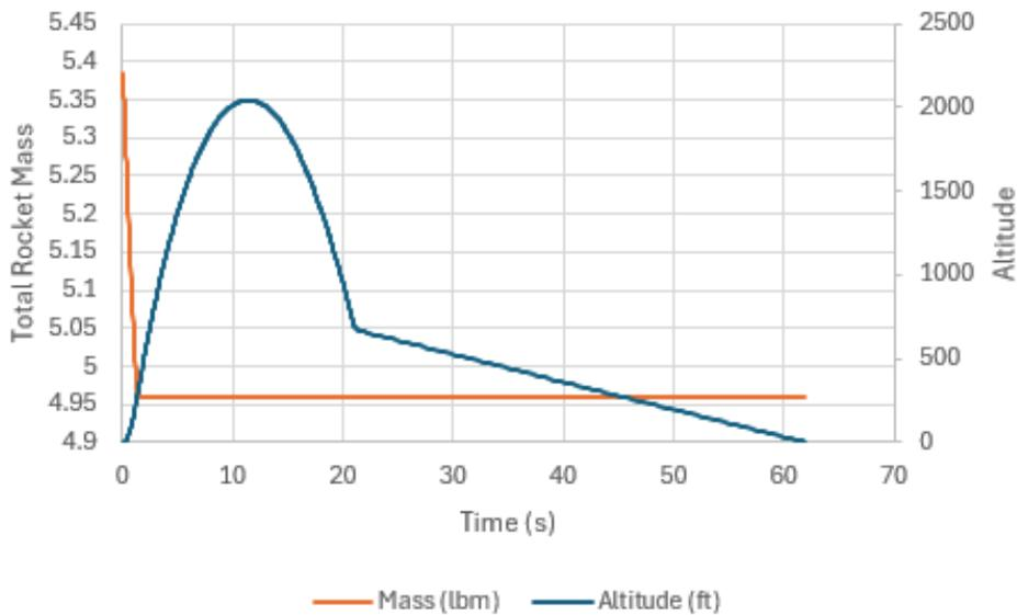
Figure 19 Initial Altitude and Total Rocket Mass Profile for I-218
