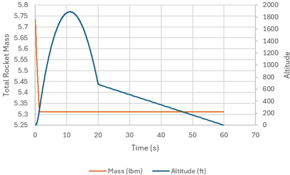
Figure 23 Final Altitude and Total Rocket Mass Profile for I-218
