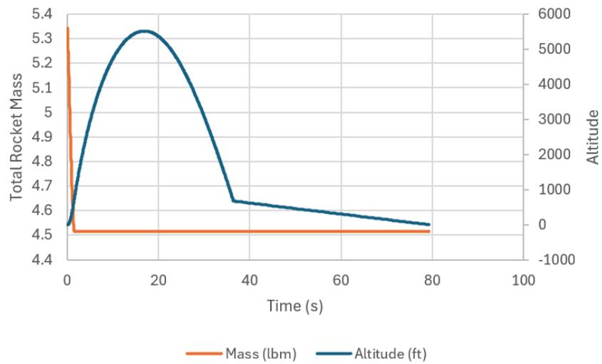
Figure 37 Second Altitude and Total Rocket Mass Profile for J-420
