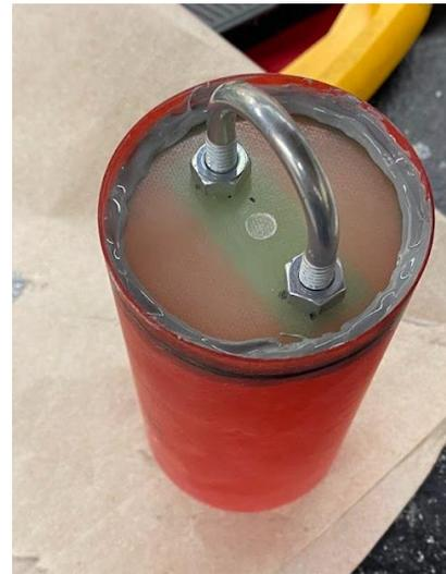
**Figure 6 Epoxied Nose Cone Coupler Bulkhead with U-Bolt Installed**
