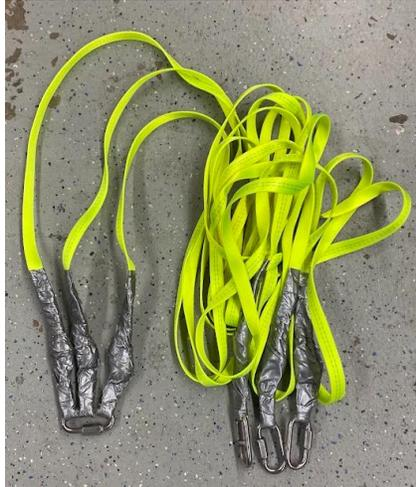
***Figure 9 Manufactured Recovery Harness***
