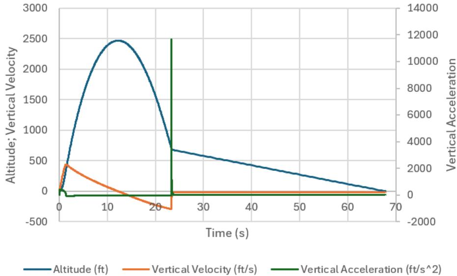
Figure 20 Second Altitude, Velocity, and Acceleration Profile for I-218
