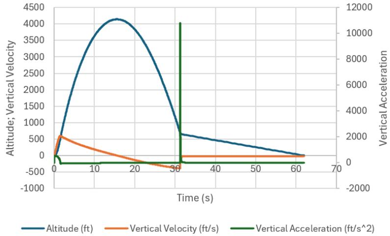
Figure 34 Initial Altitude, Velocity, and Acceleration Profile for J-420
