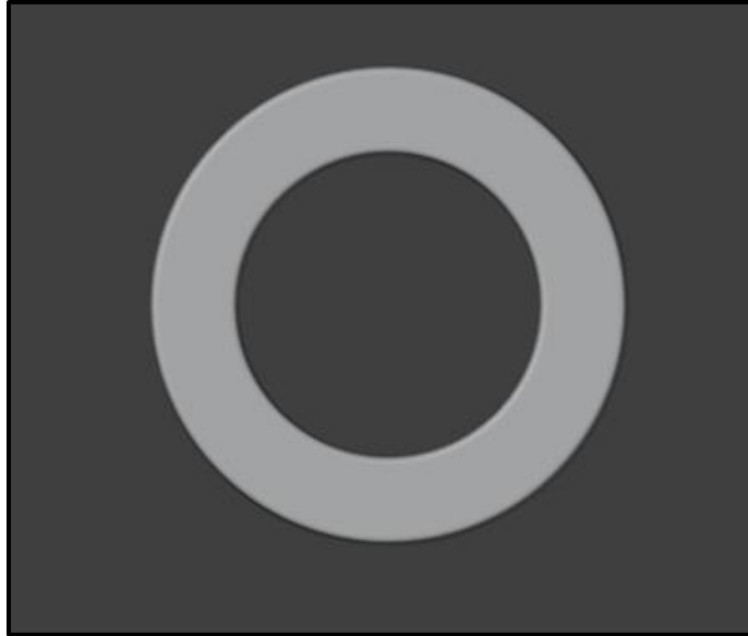
Figure 2: Grain Geometry Horizontal Cross Section
