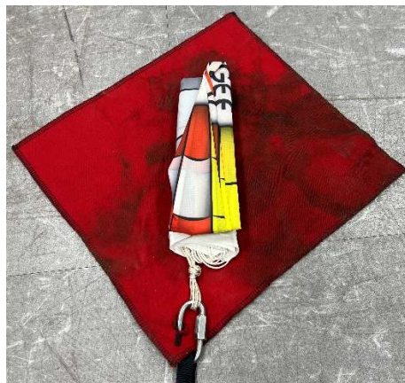
Figure 17: Folded Parachute Placed onto the Nomex Blanket
