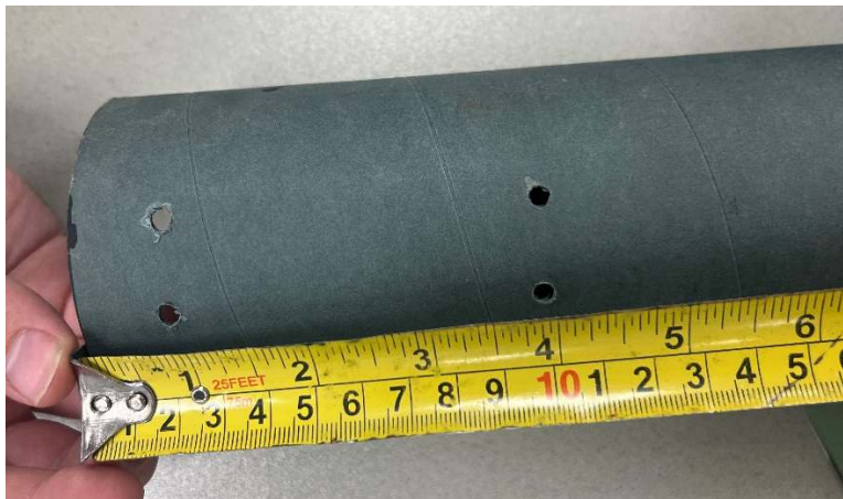
Figure 12: Placement of Fin Bracket Holes on the Aft Airframe
