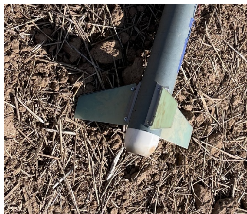
Figure 24: Broken Fin Bracket
