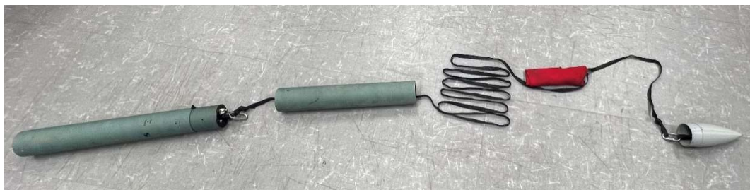
Figure 18: Completed Recovery Harness Attached to the Workshop Rocket
