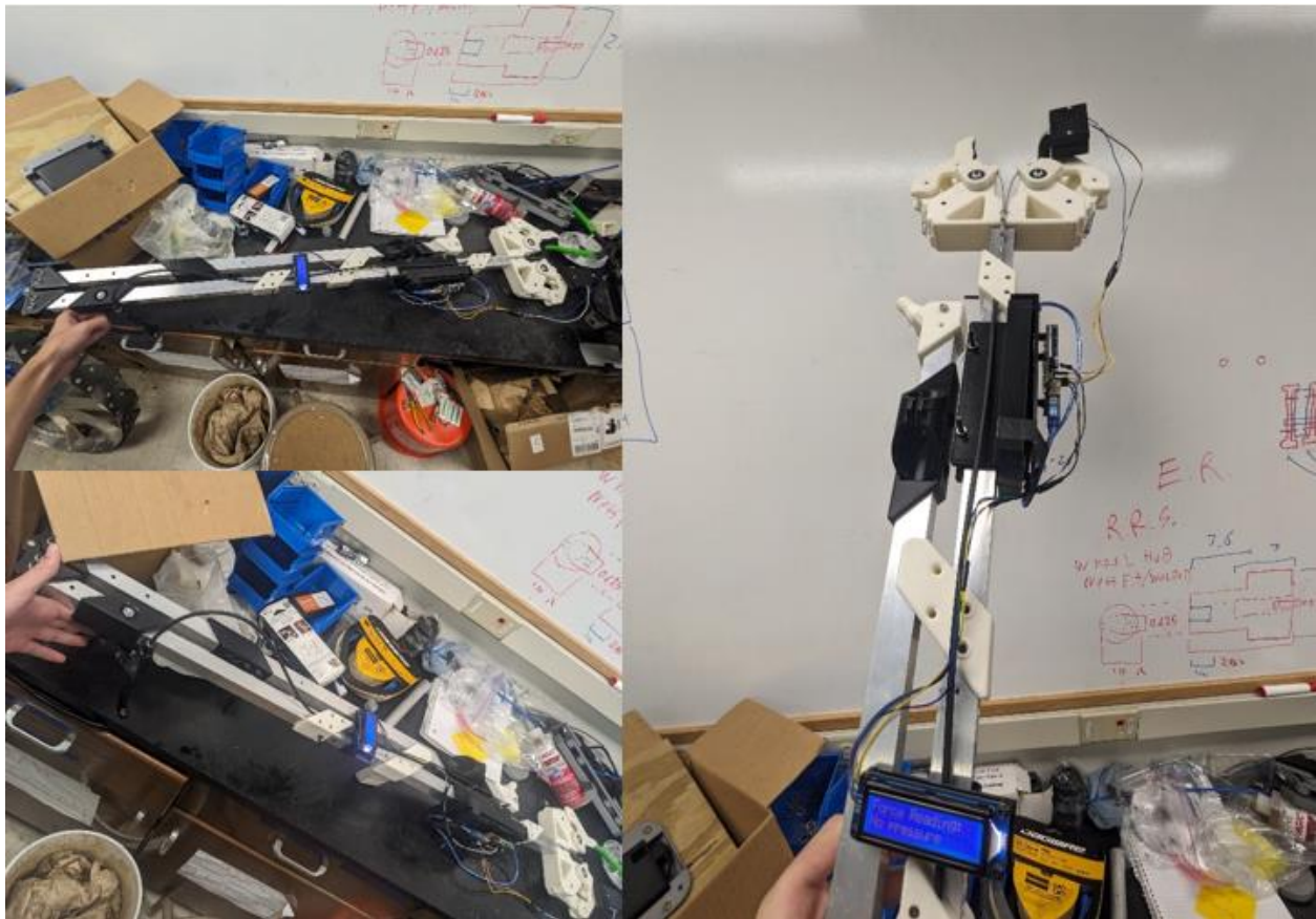
Figure 8. Force Measurement Module Installed on UAH Moonbuggy Task Tool.
