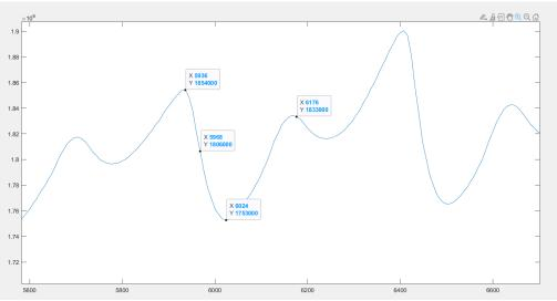
4) Calculate the characteristics that are solely based on PPG signal and compare them to what the program listed at the time of the dicrotic peak + two sample rates to account for the delay in processing caused by the filter.
