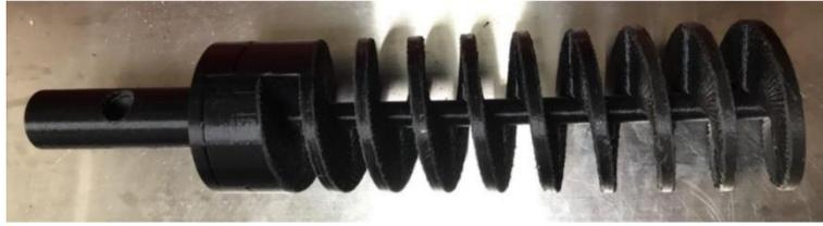
**Figure 5: 2020 Core Sampler Prototype [20]**
