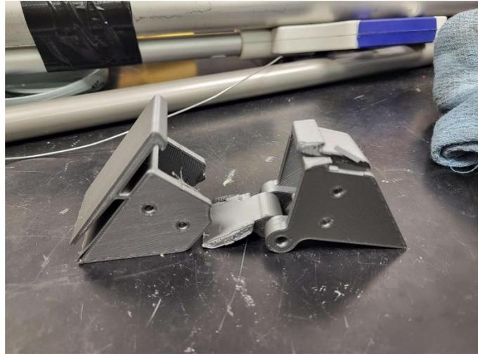
**Figure 9: First Hinge Wall Failure**
