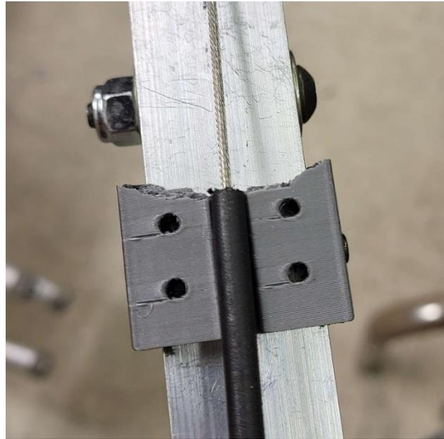
**Figure 8: Brake Cable Mount Failure**
