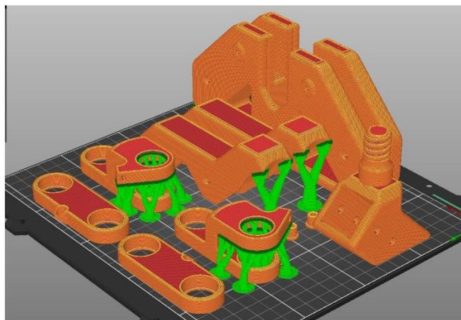
**Figure 7: PrusaSlicer Print of Gripper and Broom Components**
