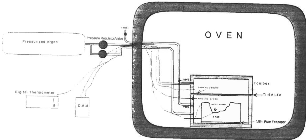
4. Rub the parting agent, boron nitride, on the mating surfaces of the toolbox and the blank.
