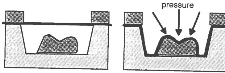
Female forming is very simple, however, the tool must be strong enough to withstand the forming pressures which may be upwards of 150psi. Expensive steel tools are often required for this type of forming.
